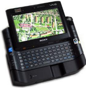
The Medic Unit in its displayed state was realized for a Sony Vaio Mini PC. The Vaio has a pressure-sensitive touch display which was used to make the application fast and easy to operate.
